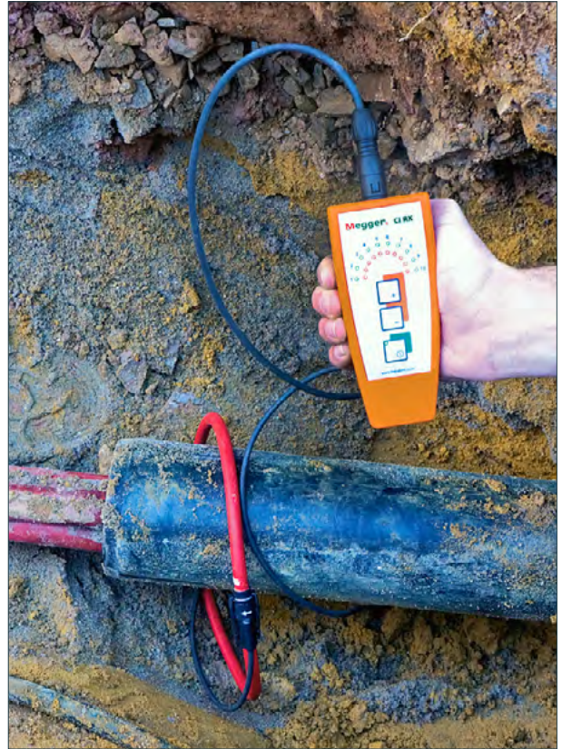
Signal pick-up: application of CI RX receiver unit and AZF flex clamp
