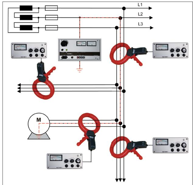
The operator follows the path of the signal current to the earth fault using inductive signal clamps (or an inductive contact sensor where cable bundling does not permit this). When the signal divides and can no longer be traced, he has found the earth fault.
