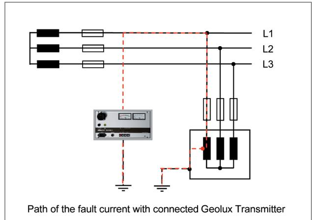
The integrated separation filter enables a direct galvanic coupling of up to 660 V AC and DC.
