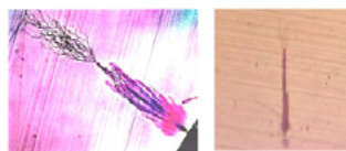
Fig. 1. Water trees of critical length can effectively be tested out by using VLF-Test methods [3].
